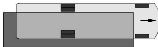
Weighing Right Rear Corner
